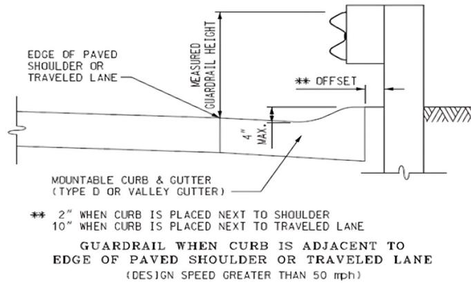
**Figure 15. Guard Rail with mountable kerb**
